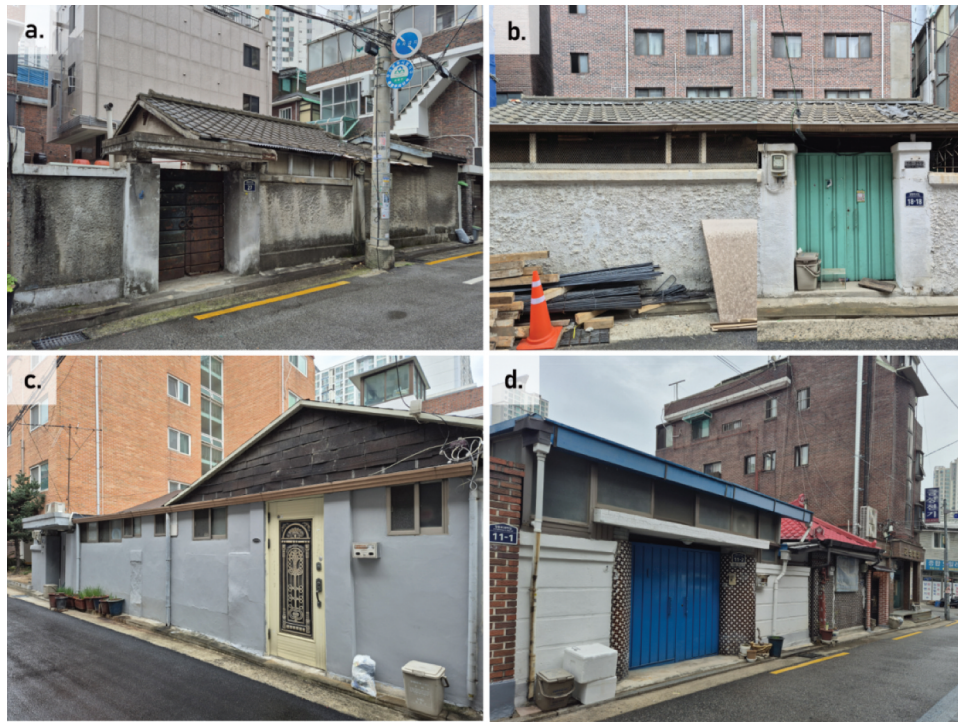
Figure 6. Remaining refugee houses in Jeongneung-dong: (a) original volume maintained with a fence; (b) eaves extended to the fence; (c) annex expanded vertically with additional entrance; (d) maximum plot usage using various materials. Source: Authors.
